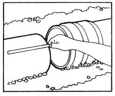
The mating areas of the spigot and socket should be thoroughly cleaned. All grease, dirt, swarf and other foreign matter should be removed from the sealing areas. If water is used in the cleaning operation, it is essential that the mating areas are thoroughly dried before the next stage of jointing is commenced.
