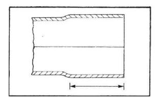
The mating areas of the spigot and socket should be thoroughly cleaned using the Watermain Cleaning Fluid provided and a clean rag or absorbent paper.
