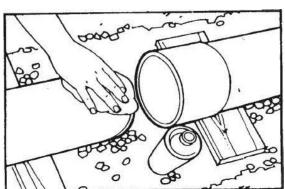
Lightly roughen the mating surfaces of the spigot and socket, using clean emery cloth or medium glass paper.
