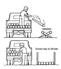
b) Where ever possible the loading and unloading of pipes should be carried out by hand. A six meter length of 10 nominal diameter PN 1 2 Watermain weighs 93 kilograms and can be carried by to men in normal site conditions.
