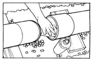
Gusing a brush of the size recommended - (see Page 33) apply an even layer of Watermain Solvent Cement to the spigot and socket mating surfaces The cement should be applied in a lengthwise direction and NOT with a circular motion. For joints of nominal diameter 3 and above, the cement should be applied simultaneously to the spigot and socket by two people.
