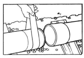
Thoroughly clean again the mating surfaces using the Watermain Cleaning Fluid provided and a clean rag or absorbent paper Ensure that all mating surfaces are clean and completely dry.
