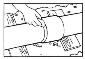
Leave the joint undisturbed for five minutes, then handle with reasonable care. N.B. See Inspection and Testing, Page 29 (Thrust Forces Section).
