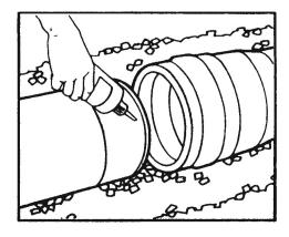
Immediately after lubrication, the spigot \_ should be brought into contact with the socket. The spigot pipe and parent joint should be accurately aligned so that axis of pipes are precisely in line. The spigot should be hand fed into the socket until resistence from the inner sealing selection is felt. Correct alignment at this stage is essential to ensure that the rubber sealing ring is not pinched or torn.
