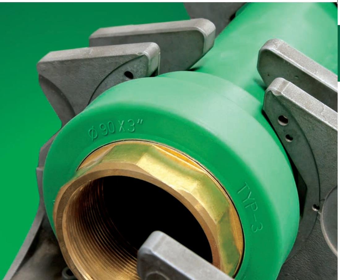
Assembly of the **RAKtherm** system is easily done by electric heating tools (threaded inserts), mounted on the **RAKtherm** welding device...a process called fusion welding.
