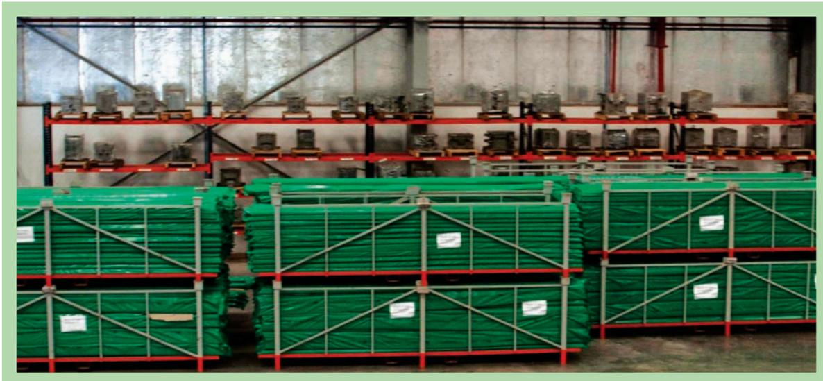
Additionally, a solid base is recommended to avoid any deformation of pipes during transportation and storage. Even though RAKtherm pipes are extremely robust it is recommended to treat the material with care.
