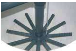
Collector arms detail
