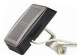
SPNODE Solar Panel Kit (optional) Height: 8 cm Length: 25 cm Width: 8 cm Controller to solar panel: 30 m maximum 1 mm 2 direct-burial wire
